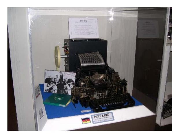
This is a picture of one of the teletypewriters used in the US/Soviet Union Hotline. The key is a one-time pad that contained on the paper spool on the left. The machine is on display at NSA's National Cryptological Museum.
